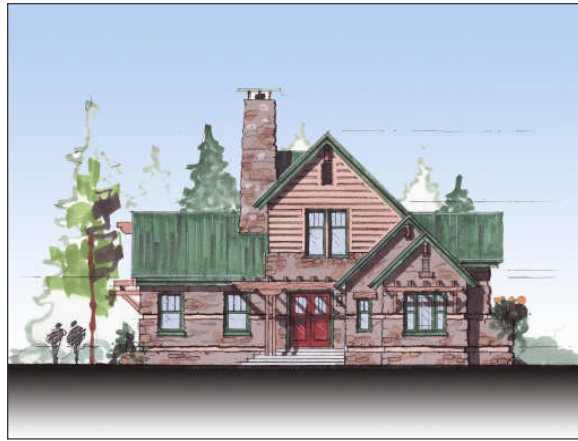
Note the tongue and groove siding
